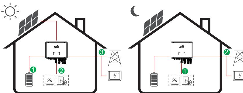
電力の流れ: PV → Battery → Load → Grid
