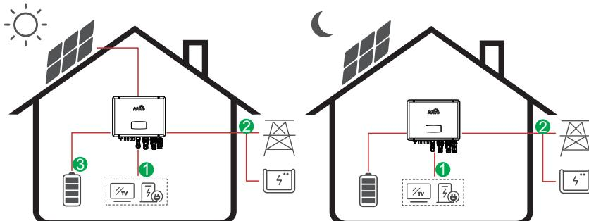
電力の流れ: PV → Load → Grid → Battery
