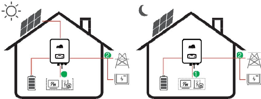
電力の流れ: Battery and PV → Load → Grid
