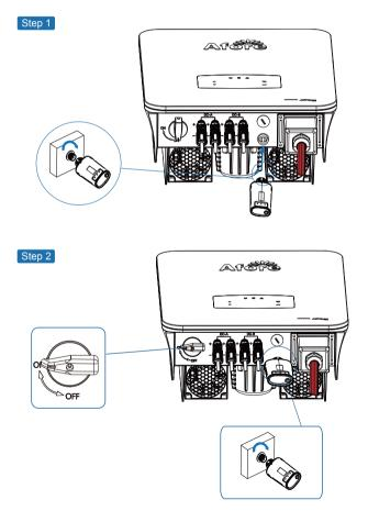
Turn on the DC switch and AC circuit breaker, and wait until the LED indicator on the monitoring module flashes, indicating that the monitoring module is successfully connected.
